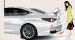
Tailgate sensor (capacitive) for 1st touchless trunk opener
